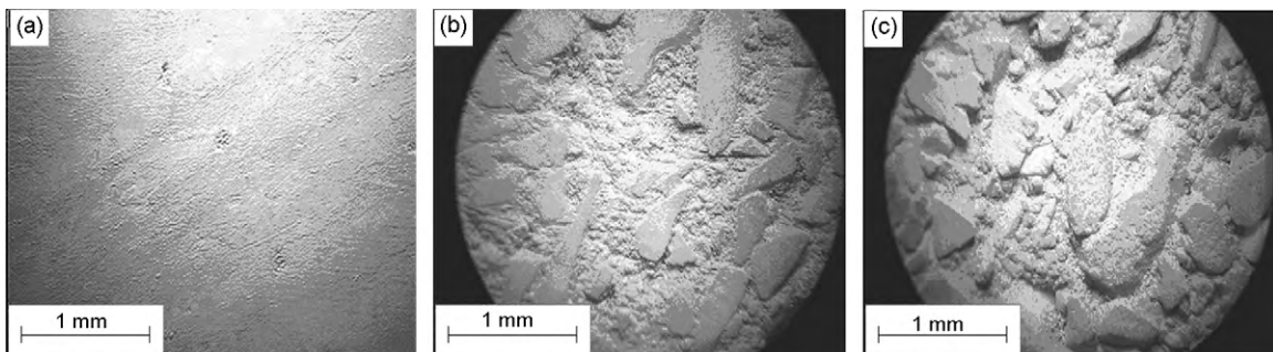
Fig. 5. Samples before and during testing: (a) before testing, (b) after 60 min, and (c) after 180 min, Fig. 6. Strength degradation (model with surface damage) versus number of cycles ( N )
